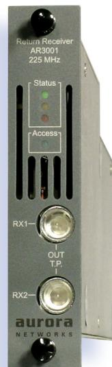
The AR3001 is a dual analog return path receiver (RPR). Its compact design (single-width module) makes it the highest density packaging in the market. It allows the operator to install up to 28 return path receivers in one 3RU chassis.
