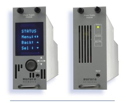
The model PS3048 is a high performance, 216 Watt power supply and controller for the model CH3000 chassis. The PS3048 accepts a nominal DC input voltage from -36 volts to -76 volts and outputs 12 volts DC to the power bus of the CH3000 mid-plane. Features include hot swap capability, load sharing for redundant operation, overvoltage, short circuit protection, and over temperature protection.
