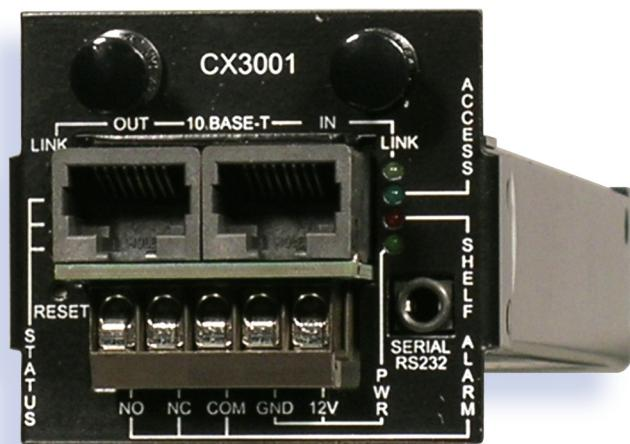
The CX3001 Communications Module supports the remote configuration and monitoring of modules in the CH3000 Chassis, monitors the chassis mid-plane alarm line (and provides contacts for connection of external alarm equipment) and provides contacts for connection of external chassis backup power. Mounted on top of any power supply module, it does not require a dedicated slot in the chassis.
