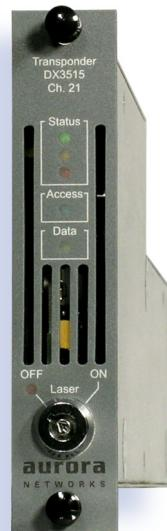
The DX3515 Digital Transponder is a high bit rate capacity (maximum 2.488 Gbps) optical converter.
