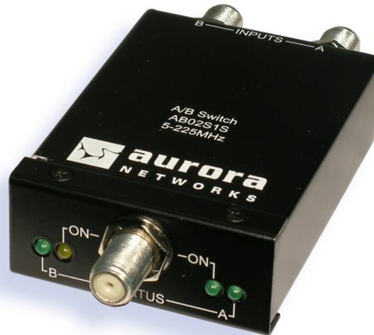
The AB02S1S-0-00 Alternate Routing Switch is an external A/B switch designed to select an RF signal from one of its two inputs and deliver that signal to its output. With a 5-250 MHz pass band, the switch provides economic and reliable support for implementing optical return path redundancy between various portions of the network where indoor receivers are deployed.
