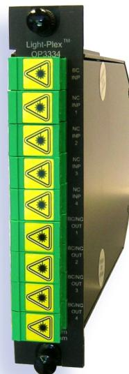
The Model OP3334 provides a single 1550 nm broadcast input port and four 1310 nm narrowcast input ports. The 1550 nm broadcast signal is split four ways for multiplexing with each of the four independent 1310 nm narrowcast signals through a minimum loss combiner, with the resulting signals passed to four broadcast/narrowcast output ports.
