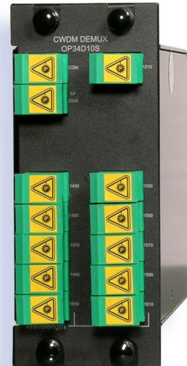
The Aurora Networks OP34D10S Series 10-channel CWDM Demultiplexers are designed to demultiplex 10 CWDM ITU-grid optical wavelengths from one fiber input, producing 10 individual wavelengths ranging from 1430 to 1610 nm (with 20 nm spacing between channels).
