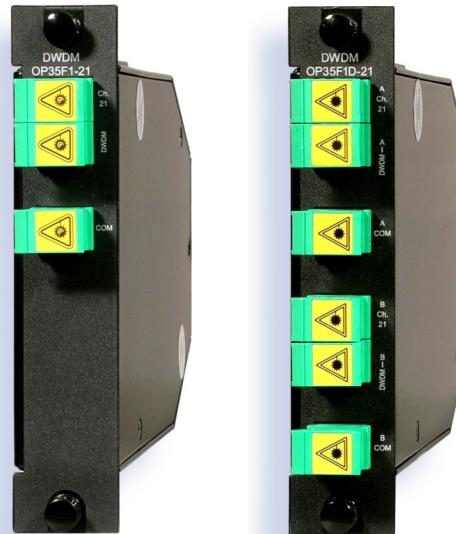
Aurora Networks OP35F1x series Single-channel DWDM Optical Filters have been designed with low insertion and polarization dependent losses. These three-port filters are used to add (or drop) a single DWDM narrowcast wavelength to (or from) a set of DWDM optical wavelengths.
