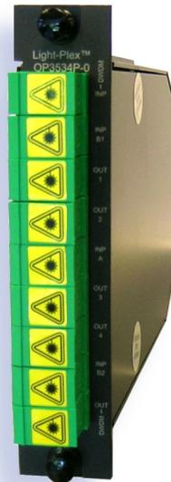
The Model OP3534 is a combined narrowcast demultiplexer and broadcast/narrowcast combiner. The OP3534 features four optical input ports (one carrying the DWDM narrowcast services and the other three for either a single four-way split or dual two-way splits of broadcast services) and five output ports (one narrowcast services pass-through port and four combined broadcast/narrowcast ports). Each OP3534 demultiplexes up to four DWDM wavelengths and is available in various wavelength combinations.
