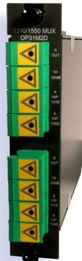
Aurora's OP31x2D family of 1310/1550 nm mux (and demux) units are provided as two independent multiplexers (and demultiplexers) in a single module and are designed to minimize the combined insertion loss of the multiplexing and demultiplexing process. Modules are provided with -20 dB test points.
