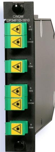
Aurora Networks' OP34F1D series Single-channel CWDM Optical Filters are three-port filters that are used to add/drop a CWDM wavelength to/from a set of CWDM optical wavelengths, where the wavelengths are 1270, 1290, ..., 1350, 1430, 1450, ..., 1610 nm on the CWDM ITU grid (*i.e.*, with 20 nm spacing). Each OP34F1D module contains two sets of identical filters (performing add/drop functions on the same CWDM wavelength).
