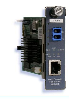
Aurora Networks' MC2401B series SMART Media Converter modules are designed to enable network planners to connect 100 Mbps twisted pair network segments to single-mode fiber optic access networks.
