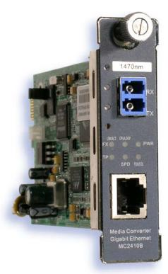
Aurora Networks' MC2410B series GbE SMART Media Converter modules enable network planners to connect 1000 Mbps twisted pair network segments to single-mode fiber optic access networks.
