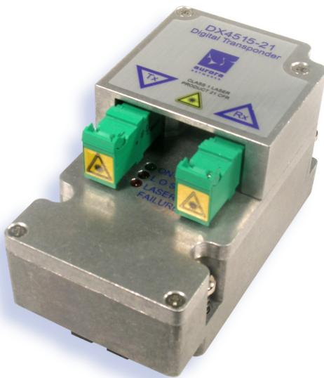
The DX4515 Digital Transponder is a component of Aurora's Integrated Digital Transport System designed to convert any communications wavelength input to a 1550nm ITU grid output. The DX4515 is a 2R type transponder. It enhances the reach of Aurora's Digital Transceiver DT4000 series modules, enabling applications that require communication through fiber spans up to 200 km long.
