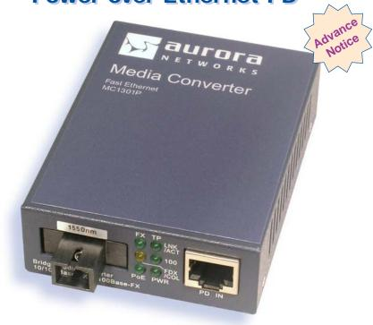
Aurora Networks' MC1301P-1550-SF Media Converter is compliant with the IEEE 802.3af Power over Ethernet standard and permits network planners to connect 10 or 100 Mbps twisted pair network segments to single-mode or multi-mode fiber optic access networks. It receives 10/100 Mbps data and power from an external PSE or PoE injector through its PD IN port and functions as a 10/100Base-TX to 100Base-FX media converter.
