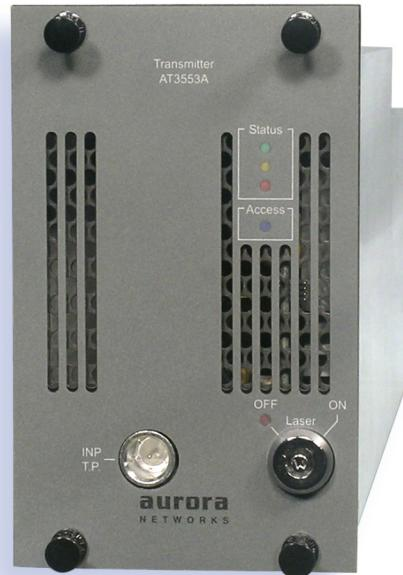
The Aurora AT3550 series high performance 1550 nm externally modulated analog transmitters are available in several optional configurations to meet various network requirements and feature minimum output power of 9.5 dBm with 14 to 18 dBm SBS suppression. The compact design minimizes rack space requirements and permits plugging the three-slot-wide, full-depth transmitter module in either the front or rear of the CH3000 3RU chassis to optimize equipment installation and operating conditions.
