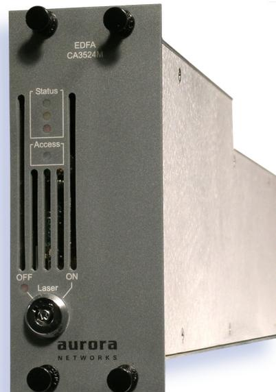
The Aurora CA3524 Broadcast EDFA is a high-output, eight port, extremely compact 1550 nm optical amplifier. Output power of 13 dBm to each of eight output ports is available in a double-width module designed for use in the CH3000 3RU chassis.
