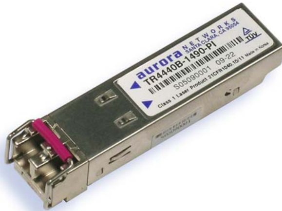
Pictured above: SFP module for 1 of 15 available CWDM wavelengths
