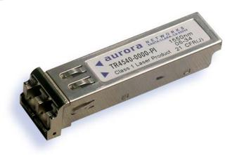
The TR4540-0000-PI 1550nm Optical Transceiver Module enable additional capabilities for high-speed communications required for Aurora Networks' digital networking products. These modules are functionally identical to the transceivers already built into many of Aurora Networks' products (e.g., DT4000 and DT5000 series optical node transceivers), but provide a flexible, plug-in means of enabling additional optional secondary ports in several of those products.
