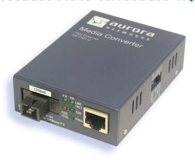
Aurora Networks' MC1301U-1310-SF Media Converter permits network planners to connect 10 or 100 Mbps twisted pair network segments to single-mode fiber optic access networks.
