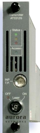
The Aurora AT3300G series 1 GHz 1310 nm Enhanced Performance Transmitters provide increased bandwidth capacity for the expanding service demands of HDTV, VoIP, VOD and high speed DOCSIS. These transmitters are ideal for broadcast and narrowcast applications for optical transport with link losses ranging from 2 to 15 dB.
