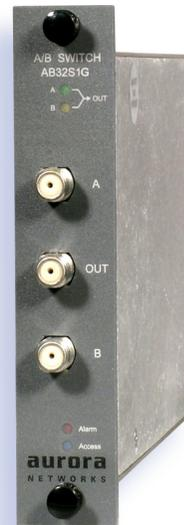
The AB32S1G-0-00 Alternate Routing Switch is an external A/B switch designed to select an RF signal from one of its two inputs and deliver that signal to its output. With a 46–1002 MHz pass band, the switch provides economic and reliable support for implementing optical path redundancy between various portions of the network where indoor receivers are deployed.
