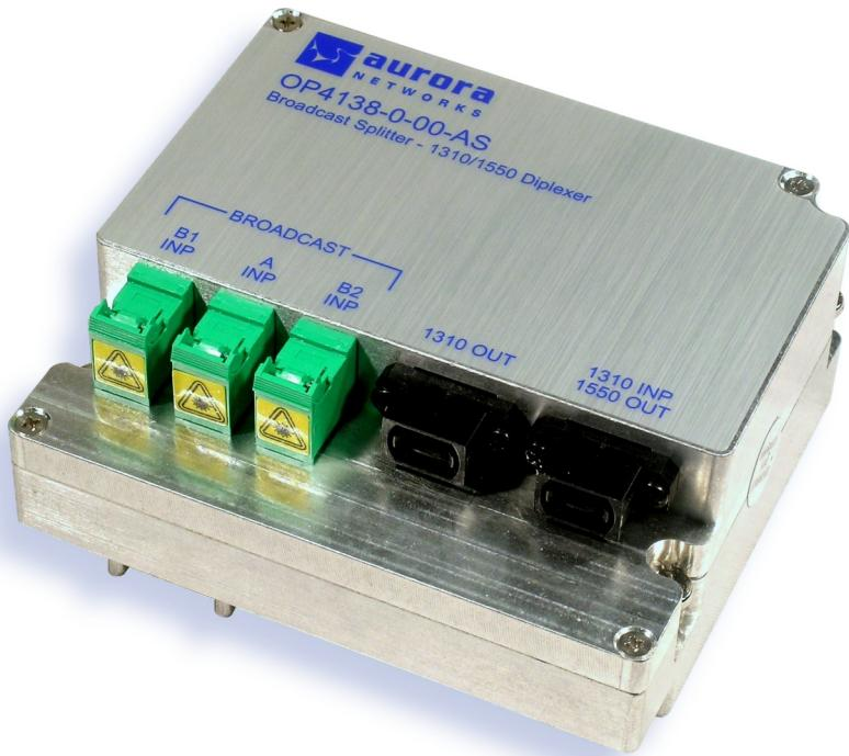
Ideally suited for FTTH applications, Aurora Networks' OP4138 plug-in module for NC4000 series Optical Nodes provides a combined optical splitter for 1550nm broadcast signals together with 1310/1550 diplex filters. This compact design, with MPO connectors, eliminates most fiber jumpers and associated losses which are normally created by broadcast splitting and/or 1310/1550 mux/demux functions.
