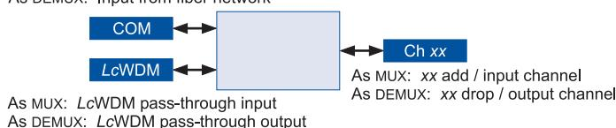
Wavelength pass-through (input or output): 1265–1357 nm
