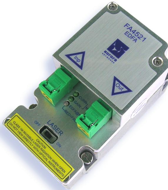
The Aurora FA4521S module is a high-output, extremely compact optical amplifier with an output power limiting function that limits the optical output power to a maximum 21.5 dBm to comply with requirements for Class 1M laser products. This high performance amplifier allows operators to use 1550 nm analog and DWDM transmitters to deliver high-quality broadcast and digital narrowcast content over significant transmission distances.
