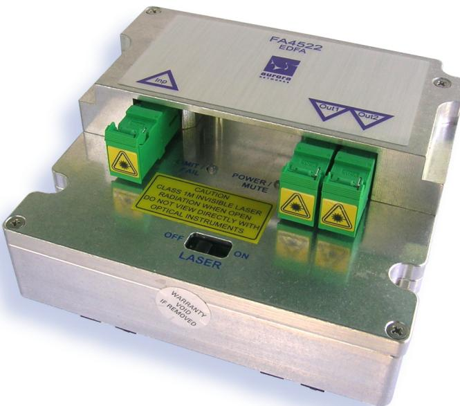
Aurora Networks' FA4522S-01 is a high-output, extremely compact 1550 nm optical amplifier with an output power limiting function that limits the optical output power to a maximum 21.8 dBm to comply with requirements for Class 1M laser products. This high performance amplifier features dual high level outputs (19 dBm per output) and allows operators to use 1550 nm analog and DWDM transmitters to deliver high-quality broadcast and digital narrowcast content over significant transmission distances.
