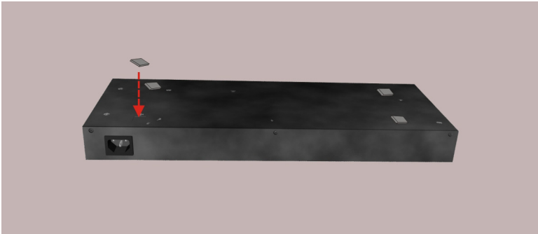
Figure 12: Attaching the Adhesive Feet
