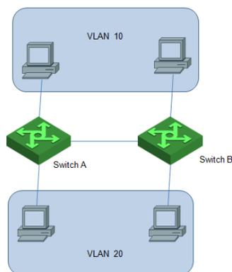
A VLAN can span across multiple GPONs, or even routers. This enables hosts in a VLAN to be dispersed in a looser way. That is, hosts in a VLAN can belong to different physical network segment.
