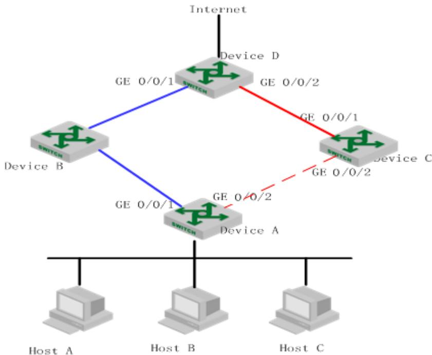
To avoid traffic interruption due to the failure of the link on which GigabitEthernet 0/0/1 of device B resides, configure a monitor link group on device B, and specify GigabitEthernet 0/0/1 as the uplink port, and GigabitEthernet 0/0/2 as the downlink port.
