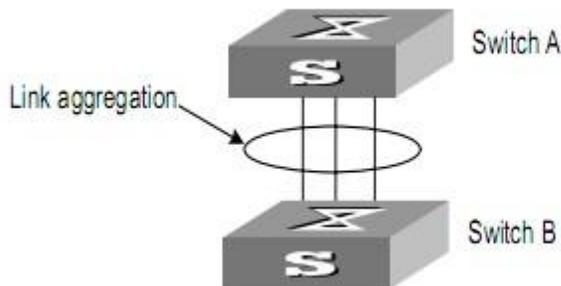
For the member ports in an aggregation group, their basic configuration must be the same. The basic configuration includes STP, QoS, VLAN, port attributes, and other associated settings.
