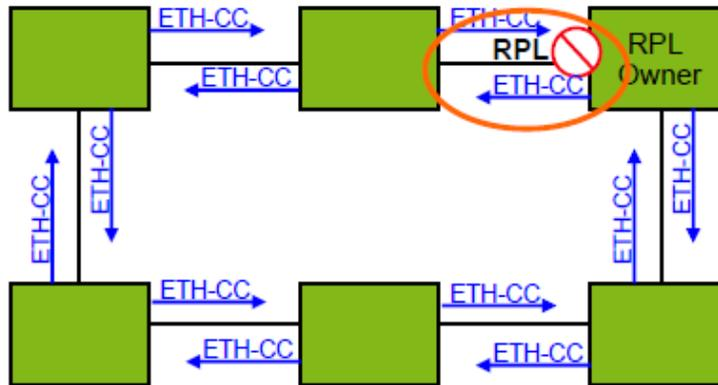
When a node on the link detects a fault, it immediately blocks the faulty node and reports the fault message (R-APS (SF)) to all the other devices in the ring. After receiving the message, all other nodes refresh the FDB. The RPL owner port receives the fault message, and the recovery port is in the forwarding state. The ERPS ring enters the protection state. As shown in the Figure:
