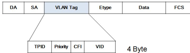
As shown in Figure 1-2, a VLAN tag contains four fields, including TPID (Tag Protocol Identifier), priority, CFI (Canonical Format Indicator), and VID (VLAN ID).
